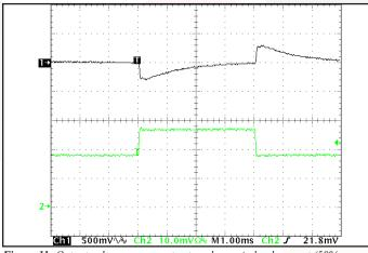
Figure 11: Output voltage response to step-change in load current (50%-75%-50% of Iout(max);  $dI/dt = 0.1 A/\mu s$ ). Load cap: 1  $\mu F$  ceramic and 15  $\mu F$ tantalum capacitors. Ch 1: Vout (500mV/div), Ch 2: Iout (1A/div).
