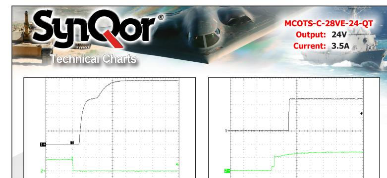
5.00 V & Ch2 5.00 V & M5.00ms Ch2 Figure 7: Typical startup waveform. Input voltage pre-applied, ON/OFF Pin on Ch 1.
