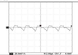
Figure 10: Output voltage ripple, Vout, at nominal input voltage and rated load current (20mV/div). Load capacitance:  $1\mu F$  ceramic capacitor and  $10\mu F$ tantalum capacitor. Bandwidth: 20 MHz. See Figure 17.
