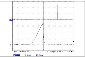
Figure 18: Load current (2A/div) as a function of time (0.1ms/div and 50ms/div) when the converter attempts to turn on into a 10 m $\Omega$  short circuit.
