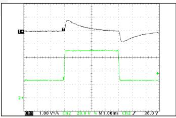
Figure 12: Output voltage response to step-change in input voltage (250V/ms). Load cap: 100 µF electrolytic output capacitance. Ch 1: Vout (1V/div), Ch 2: Vin (20V/div).
